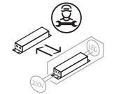
Replaceable control gear by a professional
