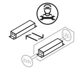
Replaceable control gear by a professional
