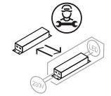
Replaceable control gear by a professional
