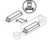
Replaceable control gear by a professional
