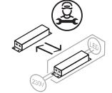
Replaceable control gear by a professional
