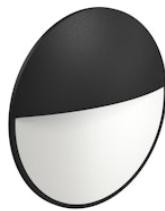
LED source included. Completed with a reflective screen. Remote electrical power supply 24V dc to be ordered separately. Optional electrical junction box (three modules, model 503) to be ordered separately. Equipped with a 250 mm protruding section of neoprene cable and a kit with crimpable connectors and adhesive heat-shrinkable sleeves that guarantee the tightness of the connection. Dimmable.
