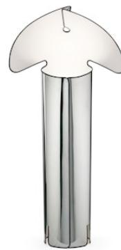
Floor lamp composed of a reflecting body in laser-cut stainless steel, finished internally with an opaque white plastic film and folded and closed via hooks formed directly from the sheet metal. A black seal in extruded TPU runs along the entire profile of the body. The internal base in painted steel is attached to the body for stability and it also supports the bulb socket. The power cable has a dimmer switch to adjust the brightness. Usable cable length: 1.9 m.
