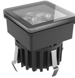
LED source included. 24V dc remote electric power supply to be ordered separately. Requires a junction box to be ordered separately. The luminaire is equipped with a protruding, neoprene, 200 mm cable with an integrated H2O STOP connection system and a wiring kit with crimp connectors and adhesive heat-shrink tubing guaranteeing the water tightness of the connection. Extra clear transparent glass. Adjustable light intensity version available upon request.
