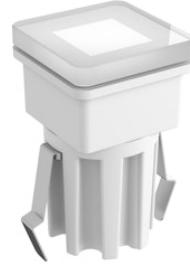
LED source included. 24V dc remote electric power supply to be ordered separately. Requires a junction box to be ordered separately. The luminaire is equipped with a protruding, neoprene, 200 mm cable and a wiring kit with crimp connectors and adhesive heat-shrink tubing guaranteeing the water tightness of the connection. Glass with opal diffuser. Adjustable light intensity.
