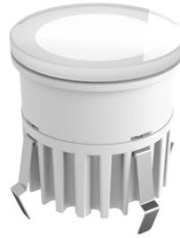
LED source included. 24V dc remote electric power supply to be ordered separately. Requires a junction box to be ordered separately. The luminaire is equipped with a protruding, neoprene, 200 mm cable with an integrated H2O STOP connection system and a wiring kit with crimp connectors and adhesive heat-shrink tubing guaranteeing the water tightness of the connection. Glass with opal diffuser. Adjustable light intensity.
