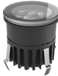
LED source included. 24V dc remote electric power supply to be ordered separately. Requires a junction box to be ordered separately. The luminaire is equipped with a protruding, neoprene, 200 mm cable with an integrated H2O STOP connection system and a wiring kit with crimp connectors and adhesive heat-shrink tubing guaranteeing the water tightness of the connection. Extra clear transparent glass. Adjustable light intensity version available upon request.
