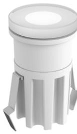
LED source included. 24V dc remote electric power supply to be ordered separately. Requires a junction box to be ordered separately. The luminaire is equipped with a protruding, neoprene, 200 mm cable and a wiring kit with crimp connectors and adhesive heat-shrink tubing guaranteeing the water tightness of the connection. Glass with opal diffuser. Adjustable light intensity.
