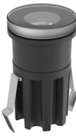
LED source included. 24V dc remote electric power supply to be ordered separately. Requires a junction box to be ordered separately. The luminaire is equipped with a protruding, neoprene, 200 mm cable and a wiring kit with crimp connectors and adhesive heat-shrink tubing guaranteeing the water tightness of the connection. Extra clear transparent glass. Adjustable light intensity version available upon request.
