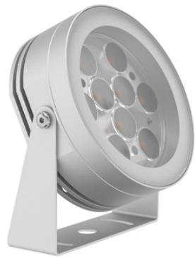
LED source included. Remote electrical power supply 24V dc ON/OFF to be ordered separately. Parallel connection. Equipped with a 2000 mm protruding section of neoprene cable and a kit with crimpable connectors and adhesive heat-shrinkable sleeves that guarantee the tightness of the connection. Fixing bracket included. Extraclear transparent glass. The metal nail for ground installation needs to be ordered separately.
