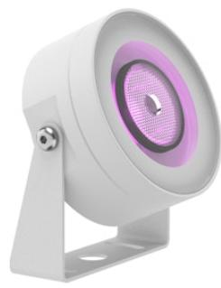
RGB LED source included. Remote electrical power supply with DMX 3chx350mA interface to be ordered separately. Serial connection. Equipped with a 2000 mm protruding section of neoprene cable and a kit with crimpable connectors and adhesive heat-shrinkable sleeves that guarantee the tightness of the connection. Transparent screen-printed glass. The metal nail for ground installation needs to be ordered separately.
