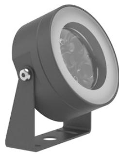
LED source included. Remote power supply 350/500 mA ON/OFF and dimmable 1-10V or DALI. Must be ordered separately. Serial connection. Equipped with a 2000 mm protruding section of neoprene cable and a kit with crimpable connectors and adhesive heat-shrinkable sleeves that guarantee the tightness of the connection. Extraclear transparent glass. The metal nail for ground installation needs to be ordered separately.
