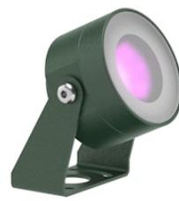
RGB LED source included. Remote electrical power supply with DMX 3chx350mA interface to be ordered separately. Serial connection. Equipped with a 2000 mm protruding section of neoprene cable and a kit with crimpable connectors and adhesive heat-shrinkable sleeves that guarantee the tightness of the connection. Sandblasted screen-printed glass. The metal nail for ground installation needs to be ordered separately.
