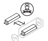
Replaceable control gear by a professional
