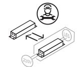
Replaceable control gear by a professional
